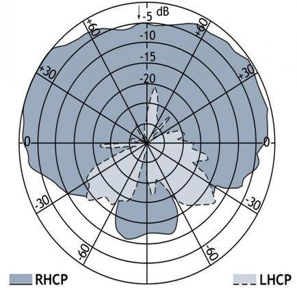
COURBE DE REPONSE TYPIQUE ET DIAGRAMME DE RAYONNEMENT POUR LA PARTIE GPS (1575 MHz)
