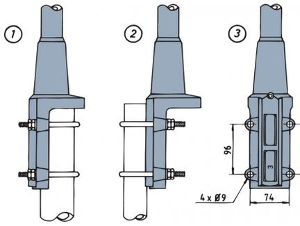
1 M, t Di, min. = 32 mm M, t Do, max. = 65 mm 2 M, t Do, max. = 42 mm M, t Do, min. = 27 mm
