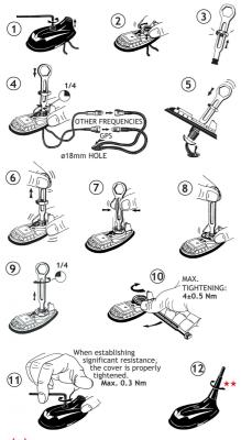
The whip should always be dismounted during car wash. Do not use sealer on rubber gasket or other places.
