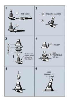
PLEASE NOTE: When tightening the revolving nut (see picture 4), special care must betaken to keep the spanner in the correct position.
