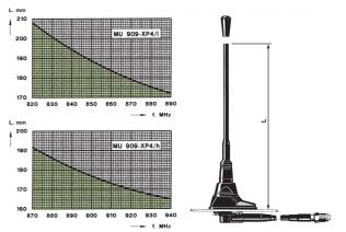
The antenna should always be tuned using an SWR-indicating device. The cutting diagrams below serve as a guide for this procedure.
